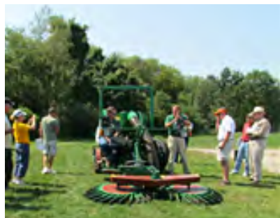
Two FACMA chestnut harvesters. BOTTOM: Tractor pulled (using PTO). TOP: Self-propelled harvester. /Photos courtesy M. Gold, UMCA.
