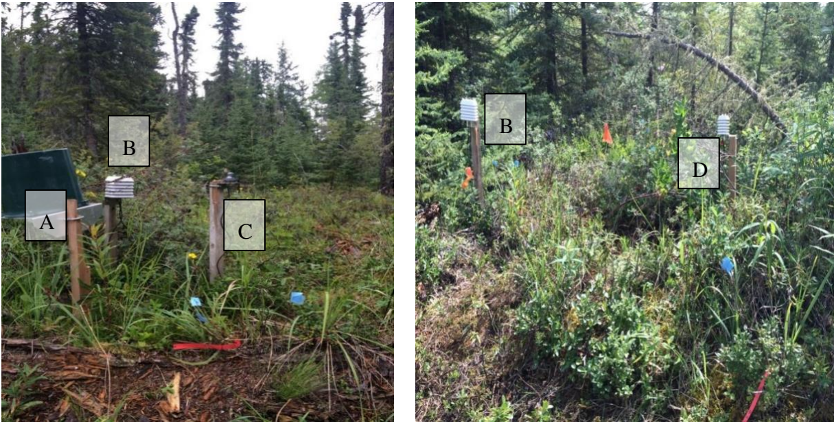
Figure 3.5. Measuring instruments installed in the selected study area. A-Automatic rain gauge WatchDog 1120, B-WatchDog data logger built with air temperature and air humidity sensors and connected to the soil temperature and moisture sensors, C-Solar radiation sensor, LightScout Silicon Pyranometer, Spectrum Technologies, D-Second backup WatchDog data logger built with air temperature and air humidity sensors and connected to the and soil temperature and moisture sensors. All equipment was from Spectrum Technologies Inc., Aurora, IL, USA.
